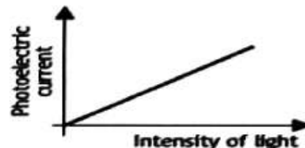
Figure 21.5: Graph of the photoelectric current versus intensity of light.
